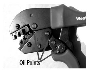
The crimp dies come pre-lubricated. We recommend that periodically you spray the dies with a light coating of silicon lubricant or WD40 to allow the crimped contacts to be removed easily and to make the dies last longer.
