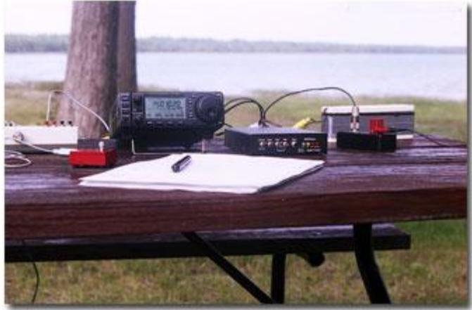
**Introduction:** In the not too-distant past, HF rigs were large and heavy. Portable operation with these transceivers (or separate transmitters and receivers) was cumbersome and difficult. Today, HF transceivers are very small and are inherently portable. (Example: ICOM IC-706 MkIIIG.) The main issues with portable HF operations have become not issues of the transmitting and receiving equipment itself but of providing power and antennas.
