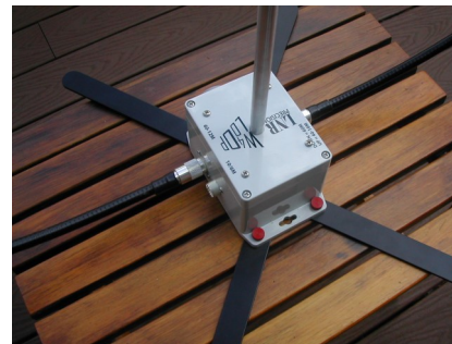
DETAIL SHOWING THE FEET DEPLOYMENT AND COAX CONNECTORS FOR THE TWO BAND SEGMENTS.
