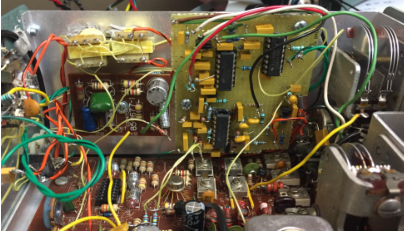
Figure 11 - Perfboard assembly is installed in the HW-8
