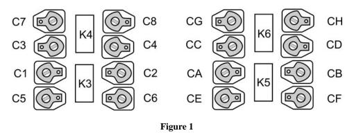
Install trimmer capacitors C1-C8 and CA-CH with their narrow ends oriented as indicated above (toward the flat side of the outline on the pc board). Each trimmer must be gently pressed down as far as it will go, but be careful not to bend the leads.
