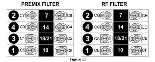
Using a small flat-blade screwdriver or tuning tool, set all sixteen trimmers so that their adjustment slots are roughly perpendicular to their flat sides (see Figure 11).
